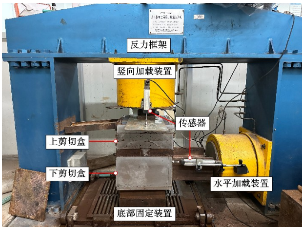
图 1 ZY50-2G 型大型粗粒土直剪、压缩试验机 Fig.1 ZY50-2G large-scale direct shear and consolidation testing machine for coarse-grained soils
