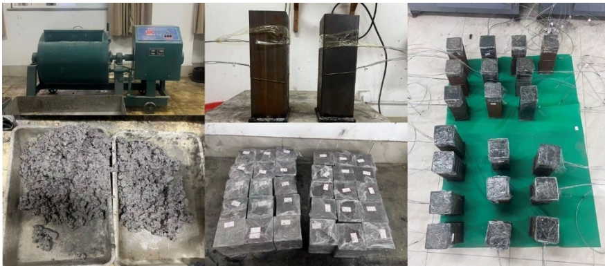
图 1 试件浇筑 Fig.1 Specimen casting
