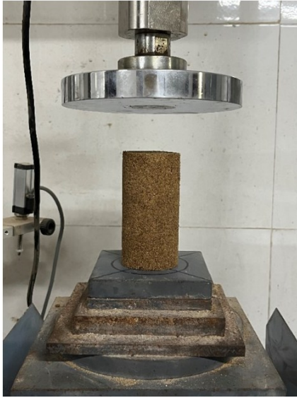
Fig. 7 UCS test on agar gum-treated sand sample
