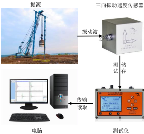
图 2 强夯振动测试设备 Fig.2 Dynamic compaction vibration test equipment
