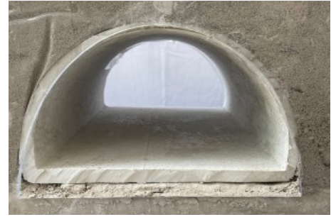
(b) 隧道扩挖后支护工况
